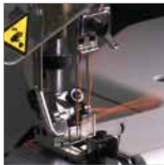
吹風 Thread Blowing
