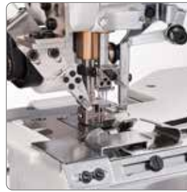
CHP (CRL 163) 氣動式下擺車縫 Pneumatic Hemming
